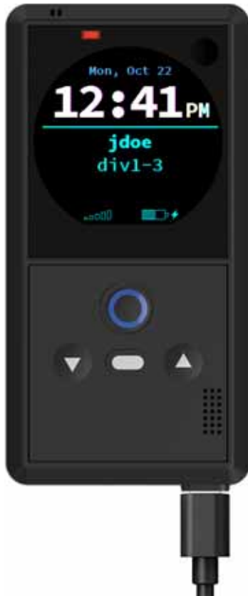
Figure 1: Device charging light with cable connected
