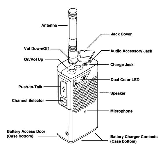
Fig. 2 Controls and Accessory Connectors
