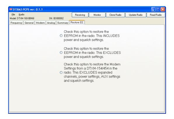
If it is desired to save the current configuration, one of the three boxes should be checked. Besides not saving a configuration by not checking any option, there are three options: Saving all parameters, saving all except the squelch and RF power level (useful is the a radio modem already has power and squelch settings with are to be retained), and an option to convert older DTXM-X54 series products to the configuration of the Series II modems.
