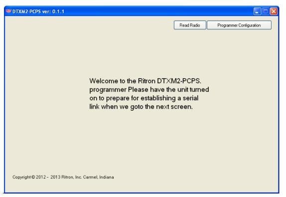
The button at the upper right is the Programmer Configuration button and is used to set the serial communications baud rate for communications between the programmer and the host computer. It defaults to 38400 baud, but can be set to other common serial rates. In addition, if the host computer baud rate is unknown, the Test Configuration button can be selected to auto-detect the baud rate. Selecting OK confirms the choice of baud rate.
