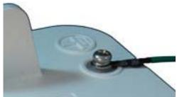
• Before the AP is mounted to a wall or pole, loosen the grounding screw (indicated by the ground symbol) on the back of the unit (see image at left and on page 6). Attach the supplied grounding wire and lug as shown and fasten the screw securely.
