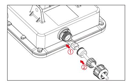
Snug the grommet assembly against the Ethernet plug and slide the collar over that.
