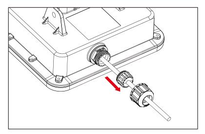
Use the screwdriver to push down the Ethernet jack's latch to release it. Unplug the jack.
