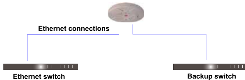
Figure 23. Switch Failover Protection
