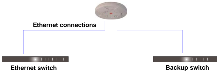
Figure 23. Switch Failover Protection
