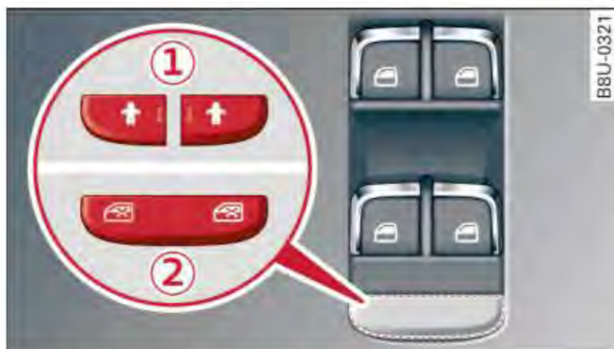
Fig. 26 Section of driver's door: controls
