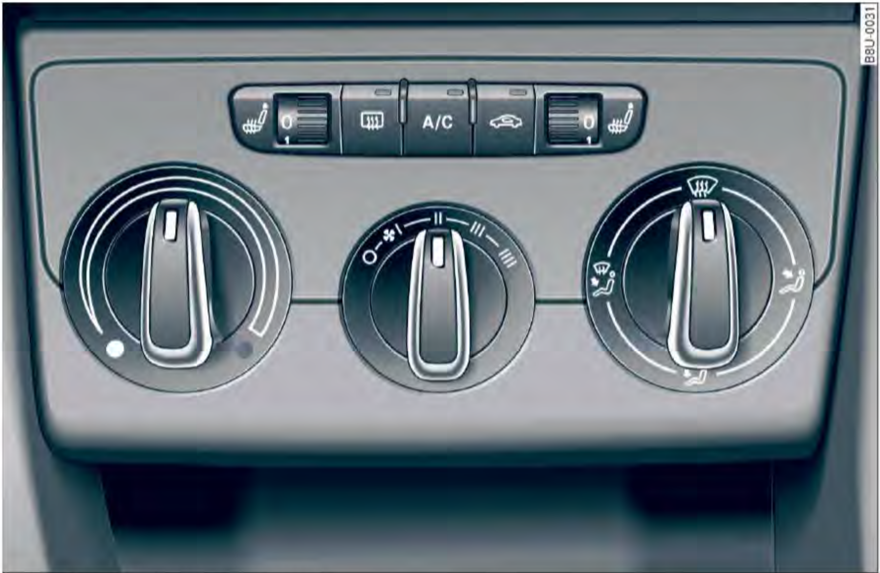
Fig. 65 Manual climate control system controls
