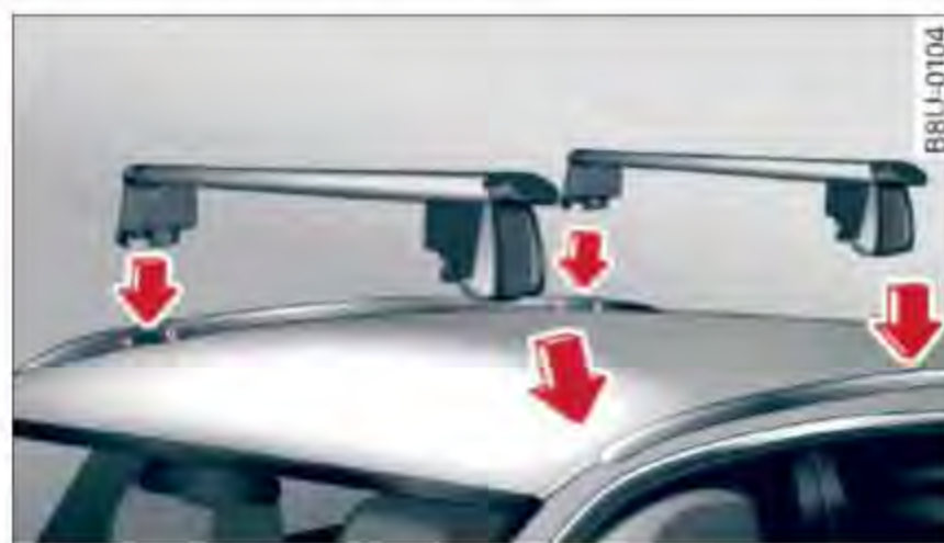
Fig. 64 Attachment points for the roof rack
