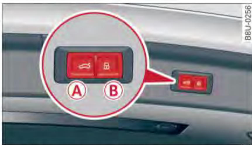
Fig. 24 Luggage compartment lid: (A) closing button, (B) lock button (vehicles with convenience key*)
