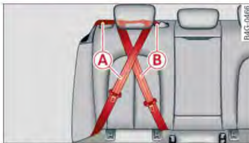
Fig. 120 Schematic overview: keep unused safety belts away from children in child safety seats. (A) - outer rear safety belt, (B) - center rear safety belt
