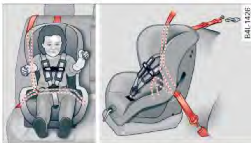
Fig. 123 Schematic overview: installation of the seat using the vehicle's safety belt system
