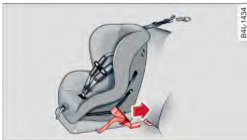
Fig. 128 Lower anchorages; proper mounting
