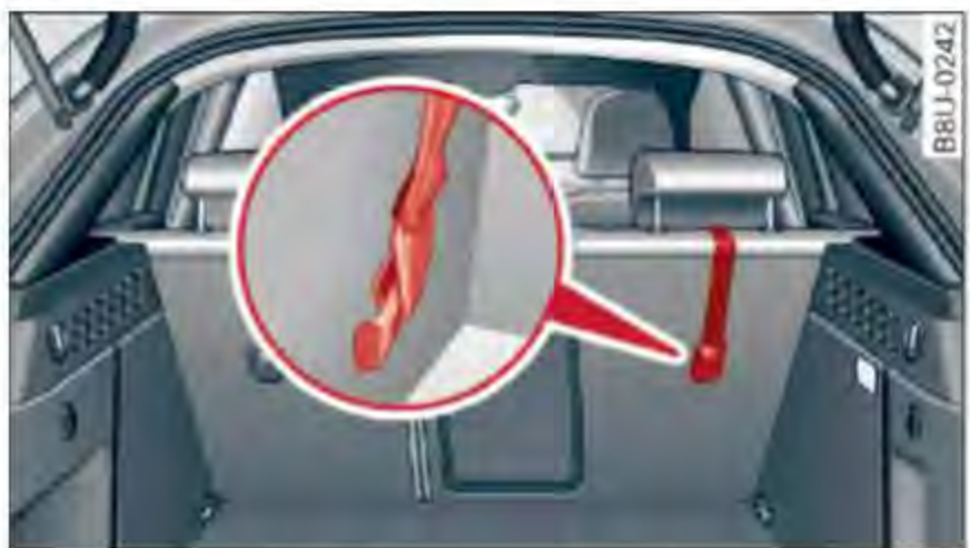
Fig. 131 Tether strap: proper routing and mounting
