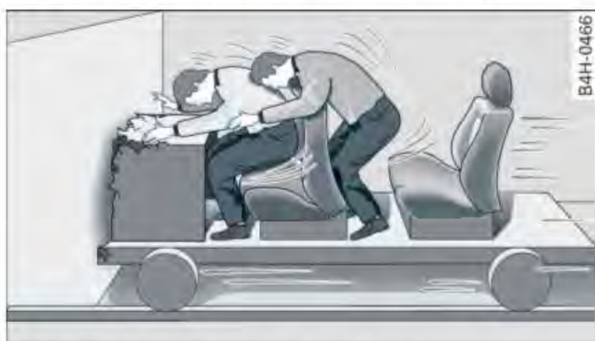
Fig. 103 The vehicle crashes into the wall
