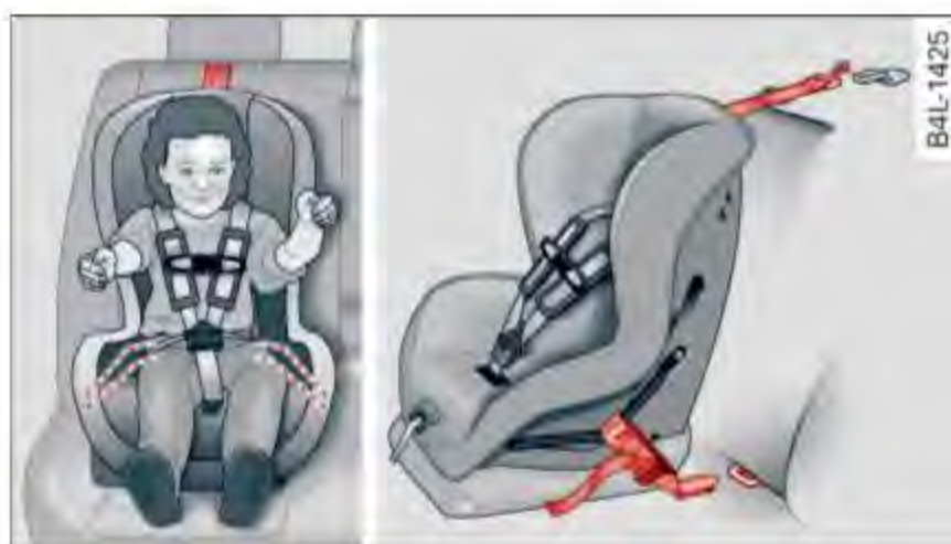
Fig. 122 Schematic overview: installation of the attachments applicable to a LATCH seat
