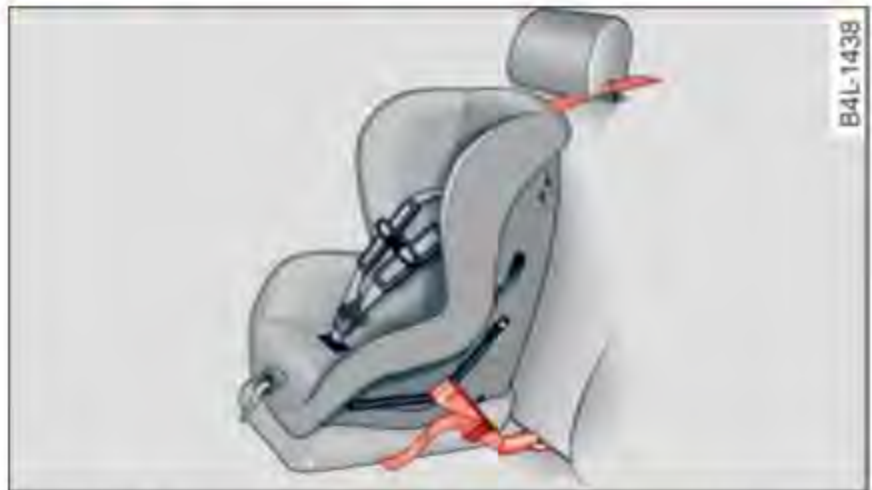
Fig. 130 Tether strap: proper routing and mounting
