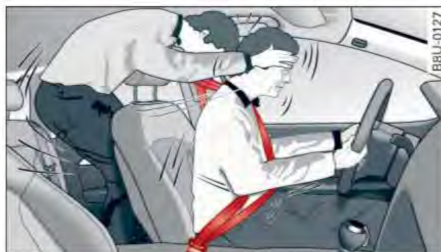
Fig. 105 A rear passenger not wearing a safety belt will fly forward and strike the driver
