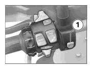
• Press button 1 to switch on the additional headlights. The indicator light for the auxiliary headlight illumin-
