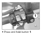
until the DTC indicator light changes its status. Immediately after button 1 is pressed, DTC system status ON and current ABS system status are displayed.
