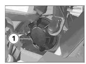
• Remove cover **1** by turning it counter-clockwise.
