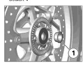
• Slip spacing bushing 1 into the wheel hub on the left-hand side.
