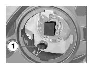
• Pull socket 1 out of the head-light housing.
