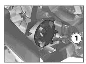
• Remove cover **1** by turning it counter-clockwise to replace
