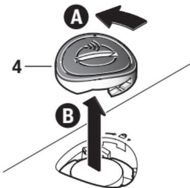
**A.** Unlock the cover of connectivity module **4** on the power tool by turning it counterclockwise with a flat-head screwdriver or a large coin. Using unsuitable objects can damage the electronics or the cover.
