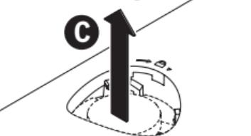
**Note:** Store the placeholder **3** of GCY30-4 in a safe place. Reinsert the placeholder again if the communications module is removed.
