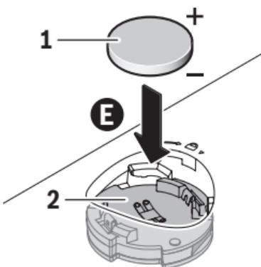
E. Insert the button/coin cell battery **1** into the GCY30-4 module **2** with the plus terminal facing upwards. It is not necessary to push in the battery.
