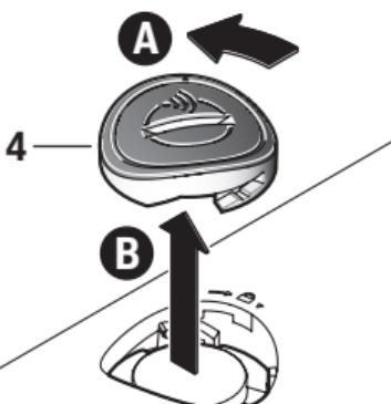
**B.** Lift the cover of connectivity module **4** and put it aside.
