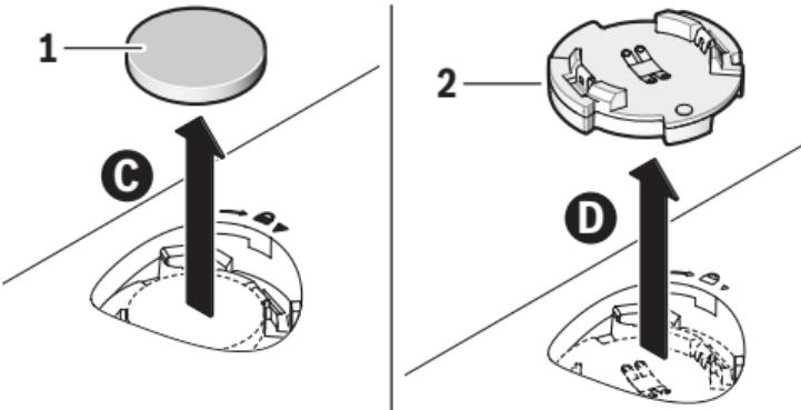
**D.** Pull out the connectivity module **2**. Do not use force to remove the module. Do not use any sharp or pointed tools.
