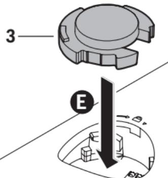
**E.** Insert the placeholder **3** into the power tool.
