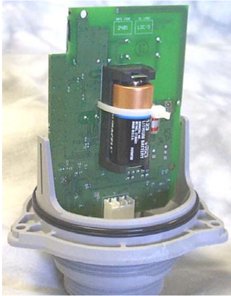
Figure 1. Radar Monitor without Cover (Replacing the Battery)
