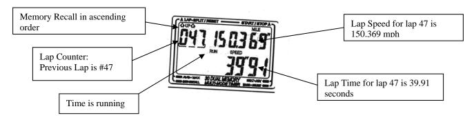
The Lap Counter will increase by one (1), each time a Lap reading is taken.
