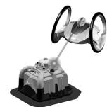
Auto-shoot the BaseStation or another robot with Roboni-i's infrared EMP Gun by pressing the Right Trigger Button on the Mobile Controller. Roboni-i will automatically take aim and shoot the BaseStation, or another robot if within range. Roboni-i should be within infrared range from the target (3 - 4 feet).
