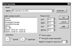
Each individual sweep is shown by when it was actually performed (date, starting time and finishing time).
