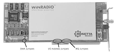
Some of the WiNRADiO IRQs can be used by other devices, for example: IRQ 3 is normally used for COM2, 5 for a sound card, 7 for an EPP or ECP printer port, 9 for a video card, 10 for a network card, 11 for a SCSI card, 12 for a PS/2 mouse port and 15 for the secondary IDE port. If you wish to use any of these interrupts, make sure that either these devices don't exist, or disable them.
