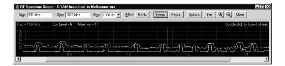
Mathematical functions can be applied to the sweeps to help find transmissions you are after. Every sweep is recorded and can be saved to a file to be viewed at a later time and different analytical functions applied to the data. Markers can also be added to the sweep, and the sweeps can be printed.
