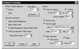
transmission is found by selecting **Record audio**, specifying a file name to record to and specifying the sampling rate and bits per sample.
