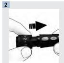
Slide the cap on until it stops by aligning the notch on the cap with the notch on the lancing device.
