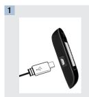
Plug the small end of the USB cable into the meter.
