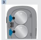
Slide the new batteries under the black tabs with the (+) side facing up.
