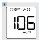
With the meter off, press or . The last stored test result appears on the display.
