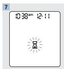
A flashing  $\Xi$  appears when there is enough control solution in the test strip.
