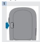
Open the battery door on the back of the meter by pushing the tab in the direction of the arrow and pulling the door up.
