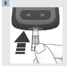
Insert the metallic end of the test strip into the meter. The meter turns on.
