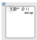
**Set-up** appears on the display with the hour flashing.
