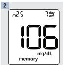
With the most recent test result on the display, press . The 7-day average appears on the display.
