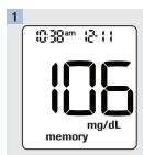
With the meter off, press or view blood glucose results stored in memory. The most recent blood glucose result appears on the display.
