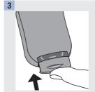
Slide the battery drawer back into position until it locks into place.
