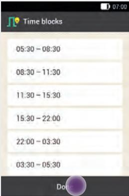
The last time block is split into two time blocks (for example, second to last time block 22:00–03:30, last time block 03:30–05:30).
