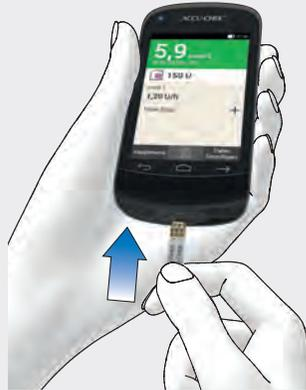
Insert the test strip into the test strip slot of the diabetes manager in the direction of the arrow. The device turns on automatically and the LED at the test strip slot lights up. If the tone for blood glucose tests is turned on, a signal is issued.
