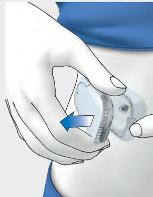
Press the flap of the infusion assembly. Remove the used micropump from the infusion assembly.
