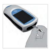
**3** Slide the new code chip into the code chip slot (as shown) until you feel it snap into place.
