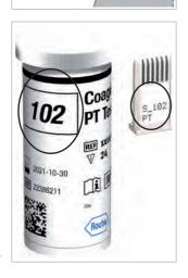
2 Check that the number on the code chip matches the number on the label of the test strip container.
