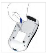
**3** Using the starshaped screwdriver contained in the kit (or another appropriate starshaped screwdriver, e.g. Torx\* size T5), remove the four screws holding the battery compartment cover in place.
