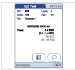
The acceptable range of results for the liquid control is displayed below the current result, along with *Pass* or *Fail*.
