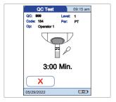
The dropper icon flashes to indicate that the meter is ready to perform the test and is waiting for the sample to be applied.
