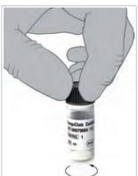
10 Swirl the bottle using a circular motion to completely dissolve all of the control plasma inside.
