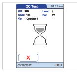
You hear a beep when you have applied enough control solution (provided the beeper is enabled). The dropper icon disappears and the test starts.
