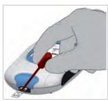
18 Apply a single drop of control solution directly from the dropper to the semicircular, transparent sample application area on top of the test strip. Do not add more control solution.
