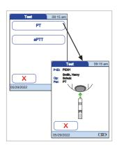
→ The barcode information appears in the patient ID field. The scanner turns off after 10 seconds, if a barcode is not scanned
