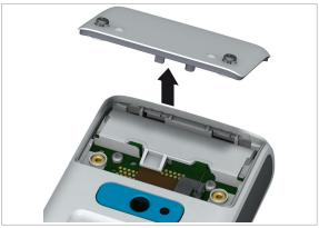
**2** Remove the battery compartment cover from the instrument. The battery is now visible and connected to the instrument by a plug.
