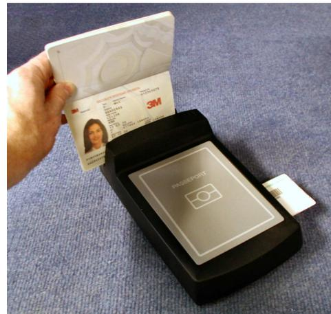
The reader incorporates has one slot for reading the codeline data off travel documents, an RFID reader is located on the main flat surface under the ePassport symbol and there are two contact smartcard slots on the right hand side of the unit.
