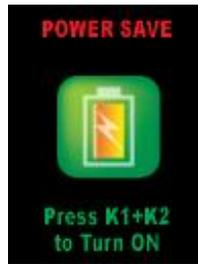
This mode saves battery power by turning off all menu screens. Pressing any remote button will display the Power Save Lock Screen.
