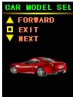
To change the vehicle display Logo, press button # 4. Press the Down Arrow to scroll thru the choices. To save the selection, press the Scroll Wheel IN.
