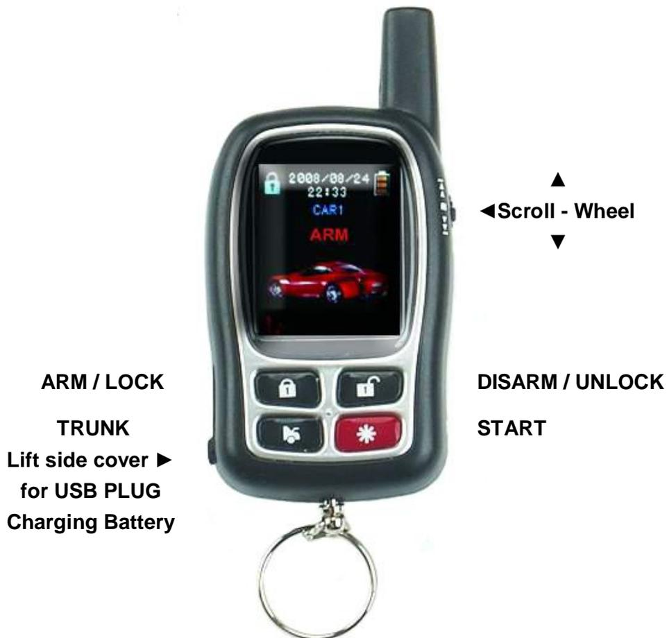
The OLED remote control will confirm everything on the display along with voice and vibration. The voice and vibration can be turned ON or OFF thru the menu choices.
