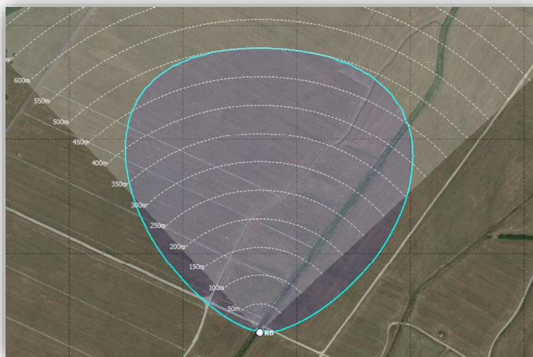
Figure 2: PSR-500 system radar detection area for human intrusion detection
