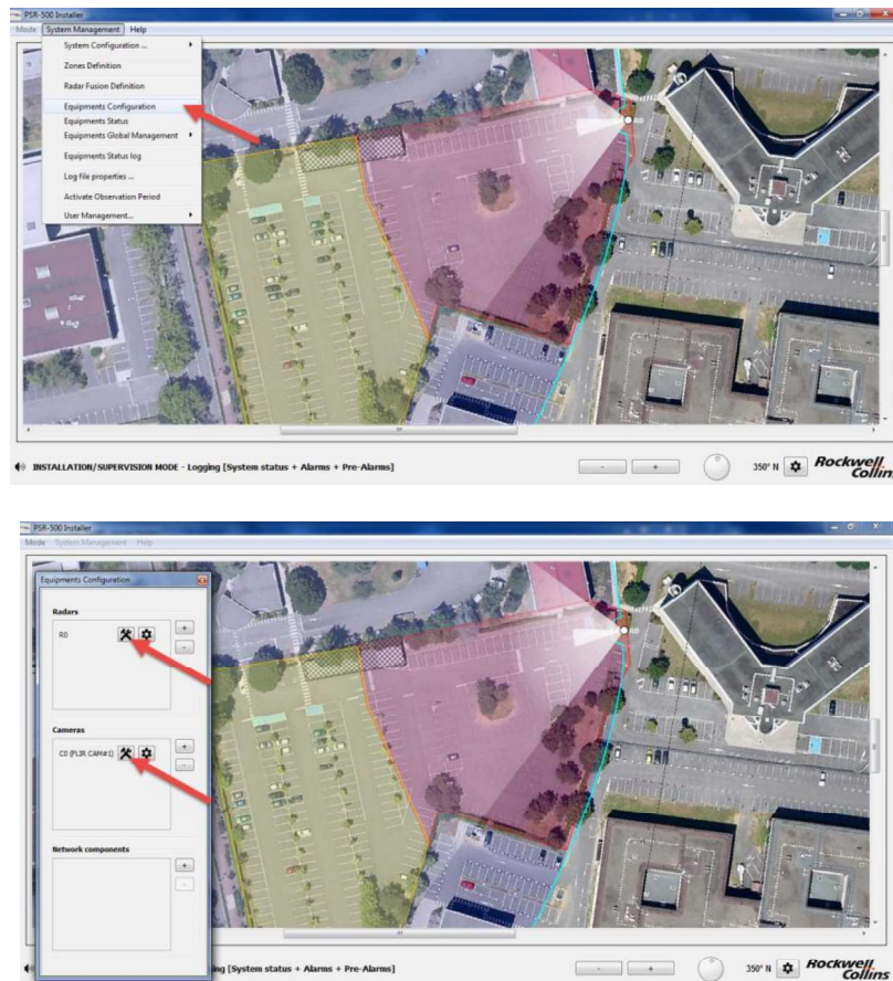
Figure 141 – Equipment installation properties update
