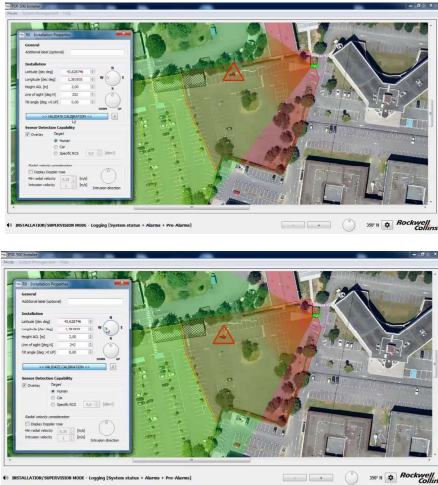
Figure 125 – Radar installation properties modification effect during radar calibration phase
