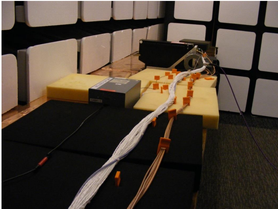
Figure 9 Cable Layout – Bulkhead Perspective
