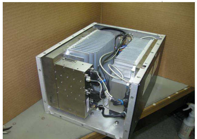
Installed RF and Power Supply
