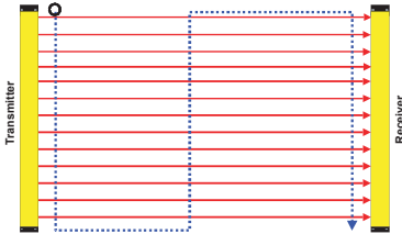
Figure 12: Correct testing of the protective field using a test rod
