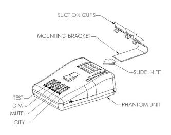
**CONTROLS:** There are 4 buttons on top of the C410, Test, Dim, Mute and City.
