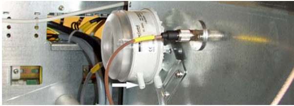
Fig. 25 Differential pressure gage without protective cap
