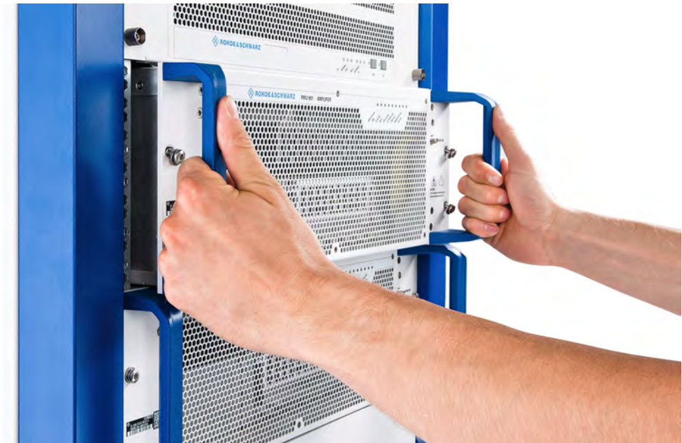
Fig. 3-11: Slide the amplifier into the rack
