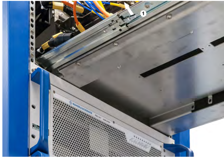
Fig. 3-14: Releasing the safety lever (left side).
