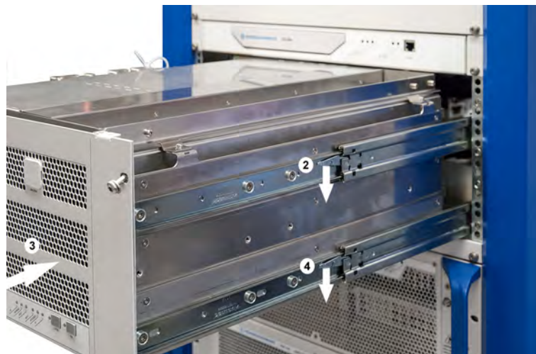
Fig. 3-15: Releasing the safety lever (right side).
