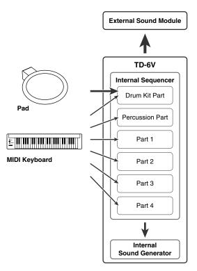
For playback, the performance data that has been recorded to the sequencer is sent to the sound module, which produces the sound. The data for each of the sequencer's parts causes the corresponding part in the internal sound module to be played. When performance data is recorded, the performance data from pads and MIDI keyboards is sent to the sequencer; the data recorded here is then sent to the sound module for playback.
