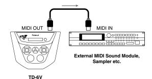
2. Match the MIDI channel to be used for transmitting data from the TD-6V and the MIDI channel that the external MIDI device will use for receiving the data.
