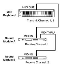
When used as a sound module, the TD-6V can receive on up to six of the sixteen MIDI channels (16 channels in GM mode). Sound modules like the TD-6V which can receive multiple MIDI channels simultaneously to play different sounds on each channel are called "multi-timbral sound modules."
