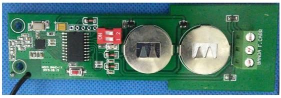
When you short circuit 1-2, Transmitter is activated and open the door. Short circuit 3-2 Transmitter is activated ,close the door. operating frequency 433.92MHz.
