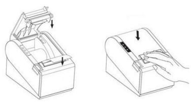
(4) Use the cutter of printer to tear off the extra paper
