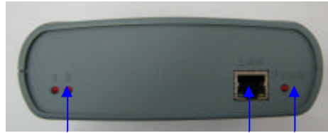
Port 1, 2 LEDS LAN-Port 3 to PC Power LED
