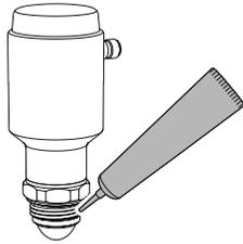
2. Mount the transmitter on the tank.
