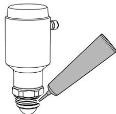
4. Mount the transmitter on the tank.
