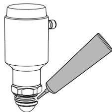
5. Mount the transmitter on the tank.
