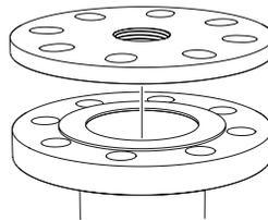
3. Tighten the bolts and nuts with sufficient torque for the flange and gasket choice.
