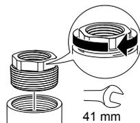
3. Apply lubricating paste on the transmitter thread.
