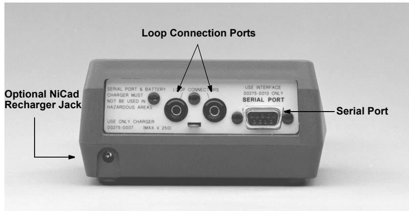
**⚠** Before connecting the 275 HART Communicator in an explosive atmosphere, make sure the instruments in the loop are installed in accordance with intrinsically safe or non-incendive field wiring practices.
