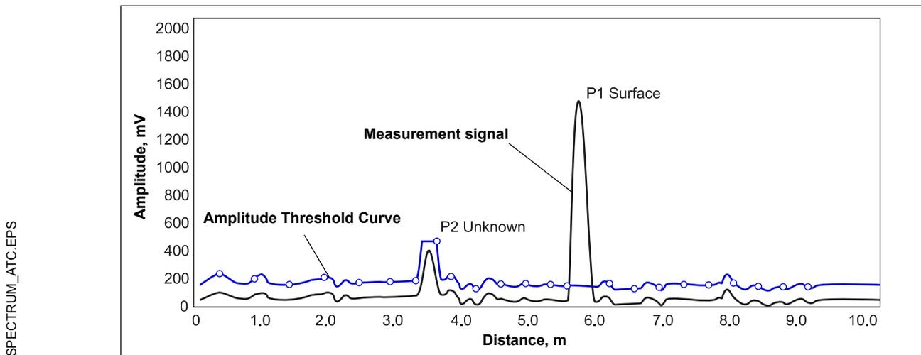
The Amplitude Threshold Curve function is available in the Rosemount Radar Master (RRM) program.
