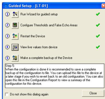
16. When configuration is finished it is recommended that the configuration is saved to a backup file. This information is useful:
