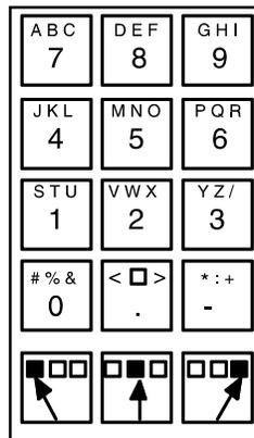
Some menus require data entry. Use the Alphanumeric and Shift keys to enter all alphanumeric information into the 275 HART Communicator. If you press an Alphanumeric key alone from within an edit menu, the bold character in the center of the key appears. These large characters include the numbers zero through nine, the decimal point (.), and the dash symbol (-).
