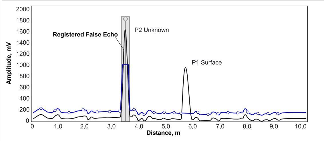
The False Echo Registration function is available in the Rosemount Radar Master (RRM) program, in the AMS Suite as well as for the 275/375 Handheld Communicator.
