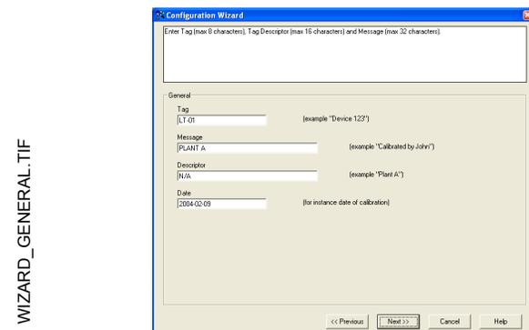
4. This window lets you enter Tag, Tag Descriptor, Message and Date. This information is not required for the operation of the transmitter and can be left out if desired. HART command: [1,4,1].
