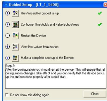
14. Restart the transmitter to make sure that all configuration changes are properly activated. It may take up to 60 seconds after the restart button is pressed until measurement values are updated.
