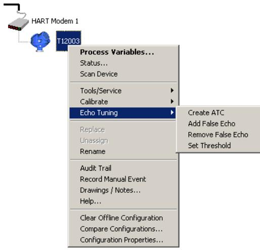
4. The Echo Tuning function offers the option to fine tune the transmitter if there are disturbing objects in the tank (see “Echo Tuning” on page 4-8):
