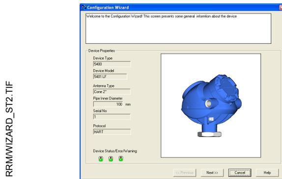
3. The first window in the configuration wizard presents general information such as device type (5400), device model, antenna type, serial number and communication protocol. Check that the information complies with the ordering information.
