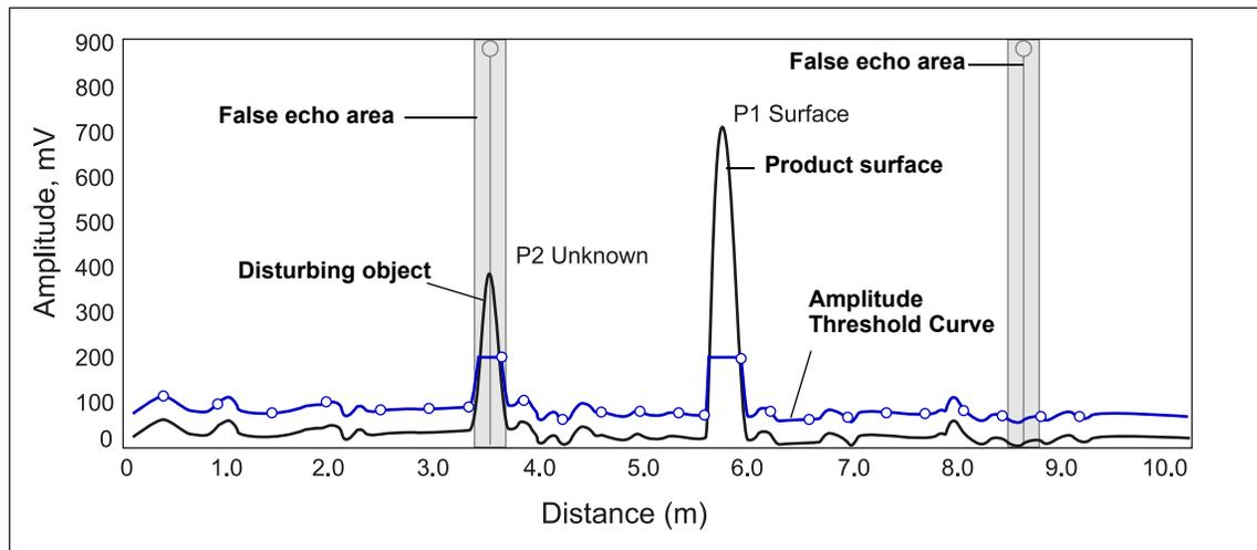
To create an Amplitude Threshold Curve (ATC) and to register false echoes click the Learn button in the Spectrum Analyzer/Configuration Mode window.
