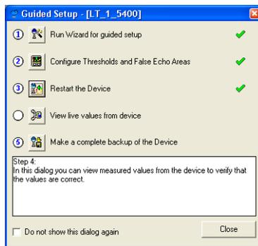
15. Step four lets you view measurement values in order to verify that the transmitter works correctly. If measured values seem incorrect, configuration settings may need to be adjusted.
