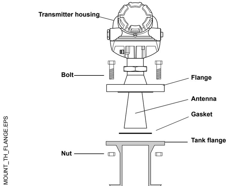
1. Place a gasket with thickness and of material suitable to the process on top of the tank flange.
