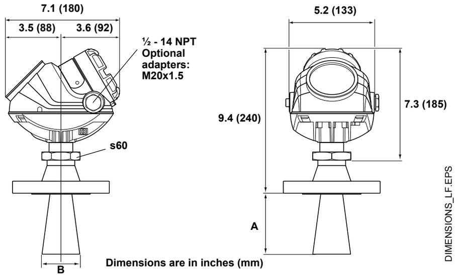
Figure A-2. Model 5402 (High Frequency version) transmitter with cone antenna.
