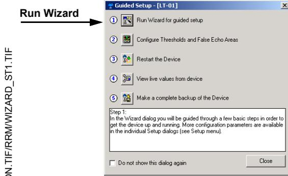
1. Start the RRM program. RRM automatically presents a list of available transmitters. Select the desired transmitter. Now the transmitter is connected and the *Guided Setup* window appears automatically.
