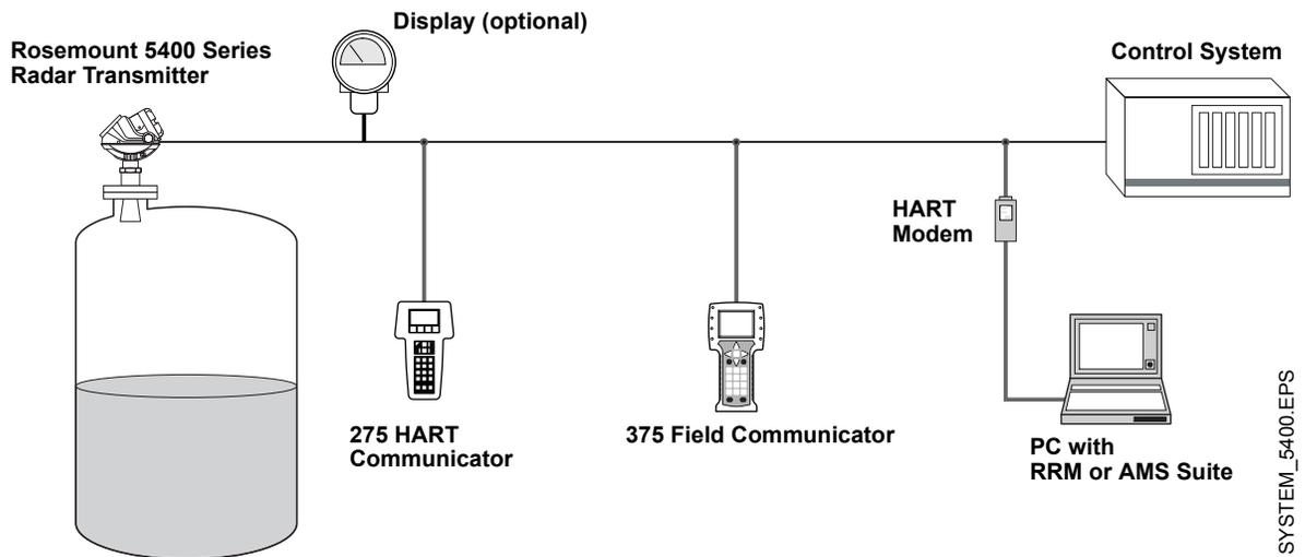
The Rosemount 5400 Series Radar Transmitter can easily be configured by using a PC and the Rosemount Radar Master (RRM) software package or via a 275/375 Handheld Communicator. RRM offers configuration and service capabilities and functions for presentation of measurement data. The transmitter is also compatible with the AMS™ Suite software which can be used for configuration.
