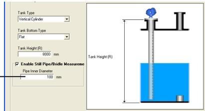
Select the **Enable Still Pipe/Bridle Measurement** check box and enter the **Pipe Inner Diameter** if the transmitter is mounted in a Still Pipe or Bridle.
