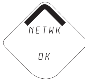
Diagnostic Button Screen 4: the device has joined a network and has been fully configured and has multiple parents. Also see "Network Connection Status Screens" on page 6-5.
