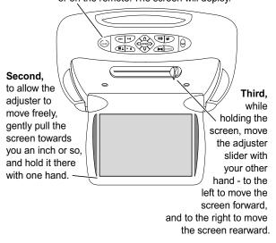
**Finally**, let go of the screen and double-check the viewing angle. You may need to repeat this process a few times to get the angle just right for your height and the height of the vehicle seats.
