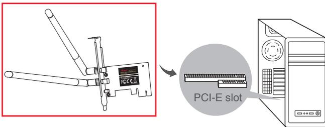
1. Screw the antennas to the Wi-Fi PCI-E adapter (RNX-N250PCEv2).
