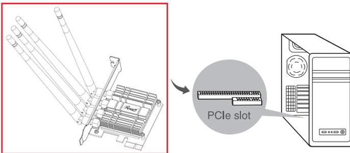
1. Screw the antennas to the Wi-Fi PCIe adapter.
