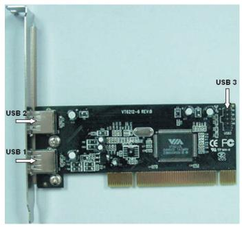
Be careful with polarity of the USB connector (USB3). Check the pin assignment while you connect the USB cable.
