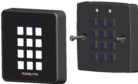
Figure 1: Removing the Top Cover
