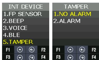
If selecting **1. NO ALARM**, even if disassembling the terminal, the alarm doesn't sound but
