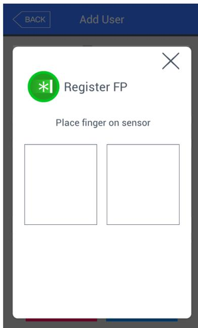
② Input fingerprint(s) referring to '1.7. Method to correctly register and input fingerprint'. Input fingerprint 2 times according to information in the screen as follows.
