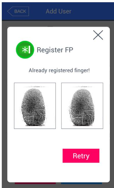
If a fingerprint is similar with an already registered fingerprint, message of "similar with an already registered fingerprint" will be displayed as shown on the left. In this case, press [**Retry**] button to start it again from the process of ② above.
