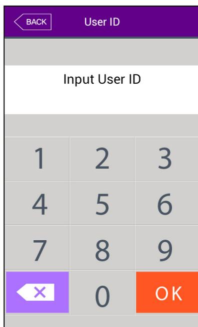
Input user ID and press [**OK**] button to display fingerprint input, face input, card input or password input screen according to Authentication Method of a user.
