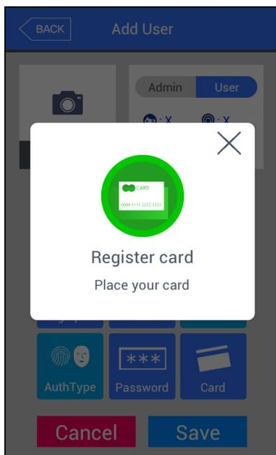
Press **[Card]** button in **[Add user]** screen to register a card. To move out without registering, press **[X]** button.
