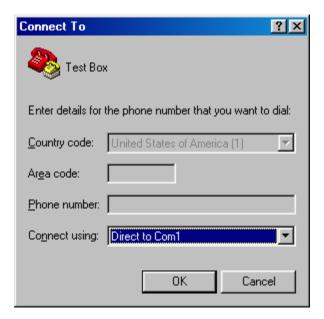
Click on the "Connect using:" list box and select either "Direct to Com1" or "Direct to Com2". Select the one that corresponds with an unused serial port connector on the computer. Click the "OK" button.
